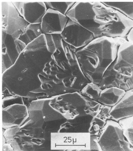
Fig. 7. Vertical shot of electrode surface polished with commercial polishing cloth, after several hundred cycles through the \text{Pb} \rightarrow \text{PbSO}_4 transition. Note residual 'hard' sulphate still remaining after three days on open circuit.
